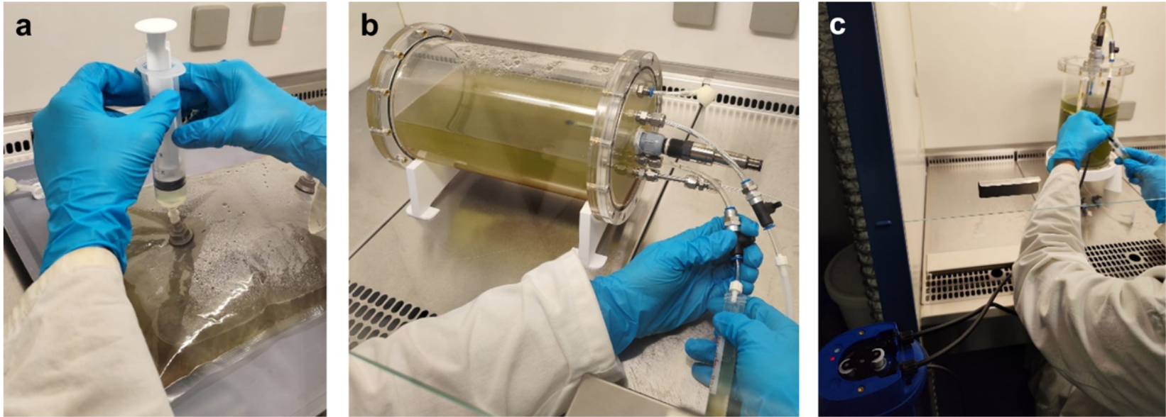
Figure 41: Sampling operations for the (a) bag, (b) rotary drum, and (c) packed bed bioreactors in the biosafety cabinet.
