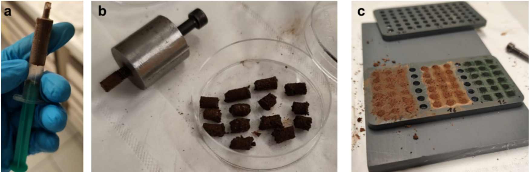
Figure 26: MGS-1 regolith pellets moulding techniques. (a) Syringe pressed, (b) cylinder pressed, (c) mould pressed.
