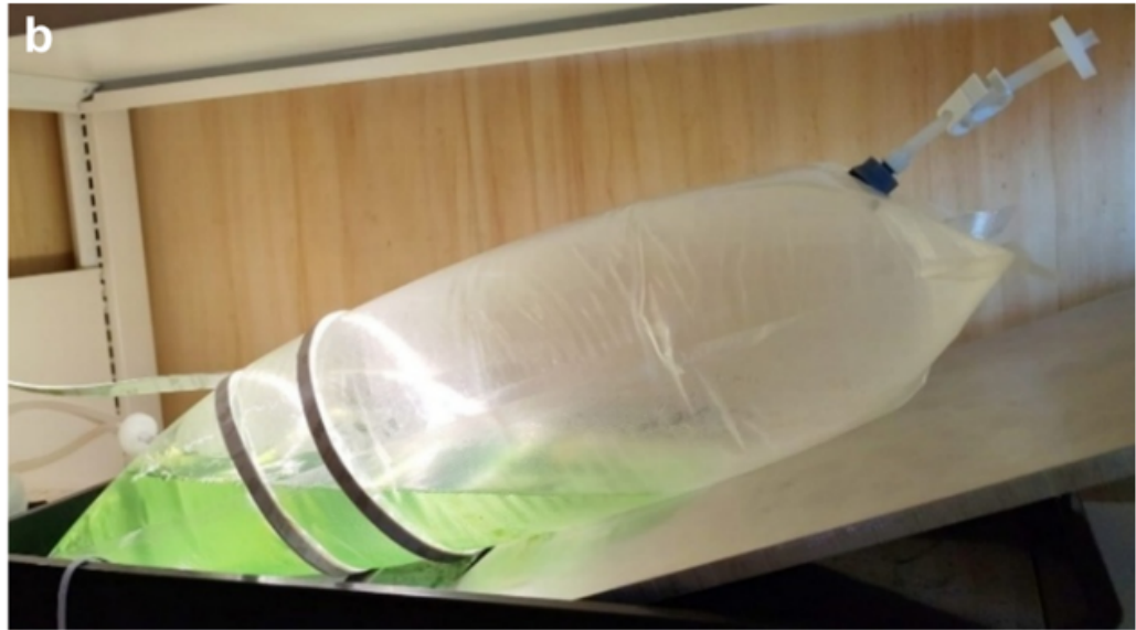
Figure 13: Tests using clear resin (a) and grey resin (b) inlets for regolith processing (0.5 L) and biomass production (5 L).
