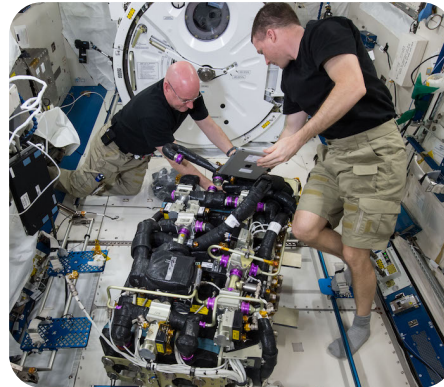
Fig 18. Carbon Dioxide Removal Assembly (CDRA) on the ISS (NASA, Wikimedia Commons)
