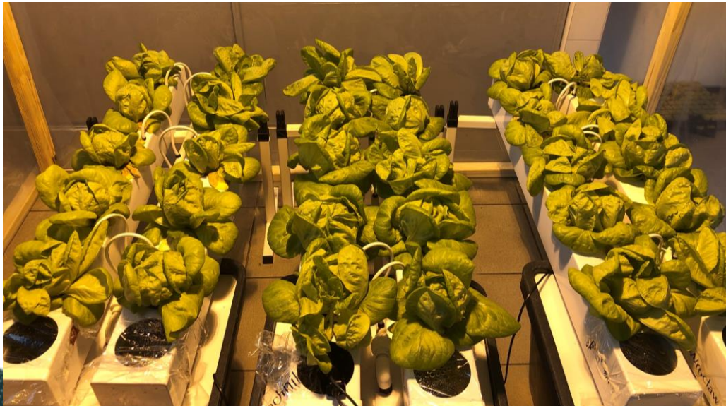
Image 3. Photo of experimental set-up of soilless cultivation of lettuce on nitrified urine.
