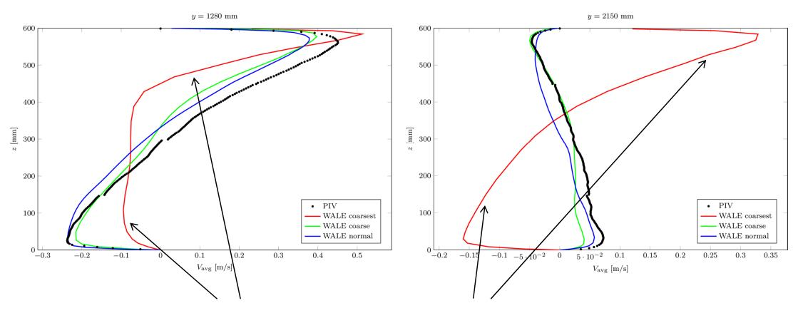
The coarsest grid is too coarse, the normal grid produces almost grid independent results
