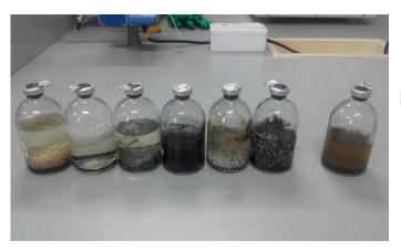
Enrichment of SAO biofilm on different support materials (nylon, zeolite, magnetite, steal, graphite, etc.)
