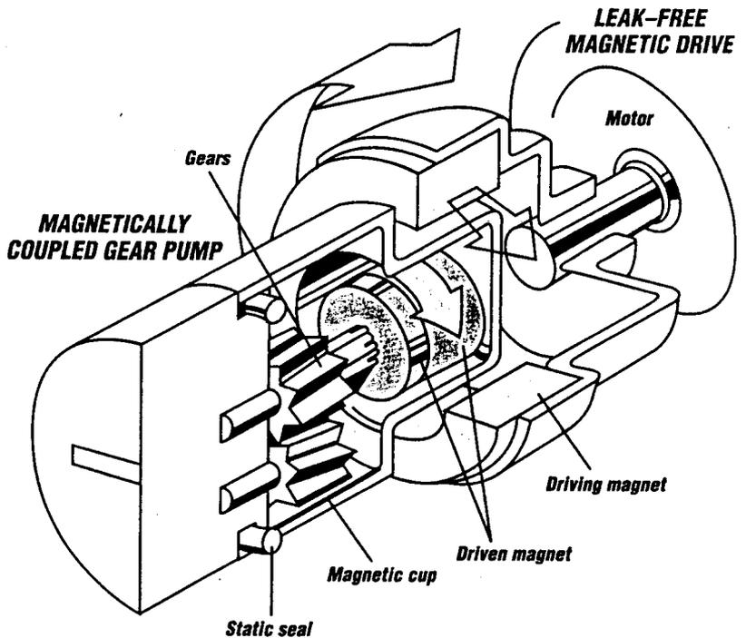
Magnetically coupled gear pumps eliminate shaft seals—ensure freedom from leaks and contamination. The conventional means of sealing pumps is by using some type of
