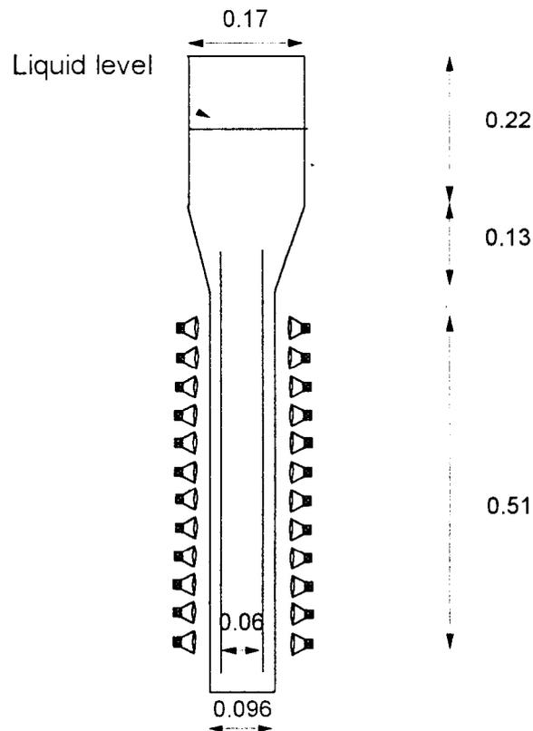
**Figure 2.** Current air-lift bioreactor configuration (reactor 1).
