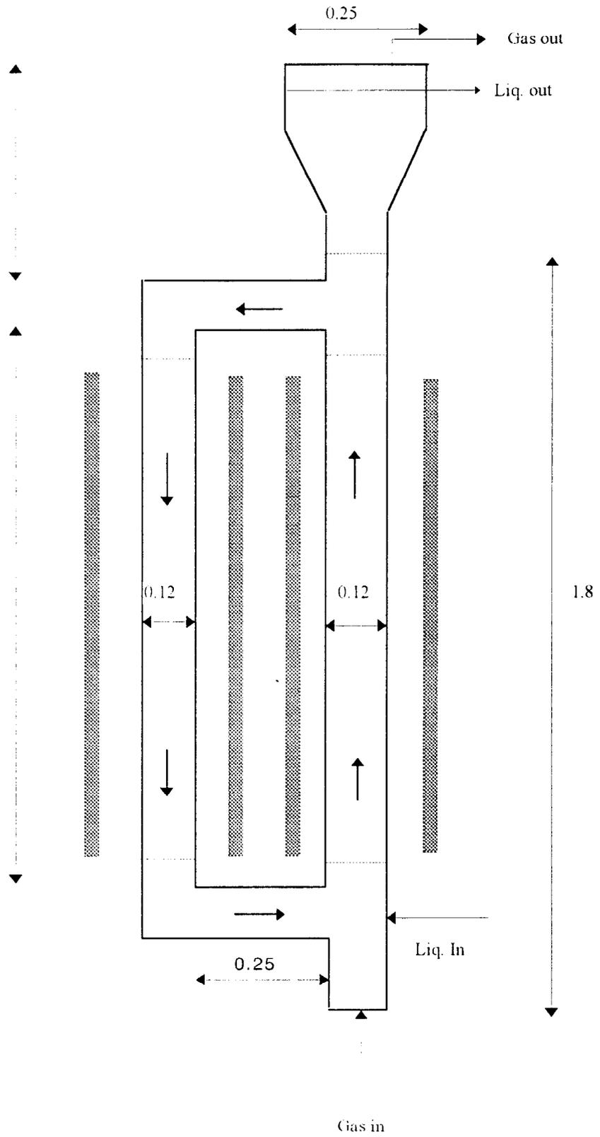
Figure 5. External loop air-lift configuration (reactor 4).
