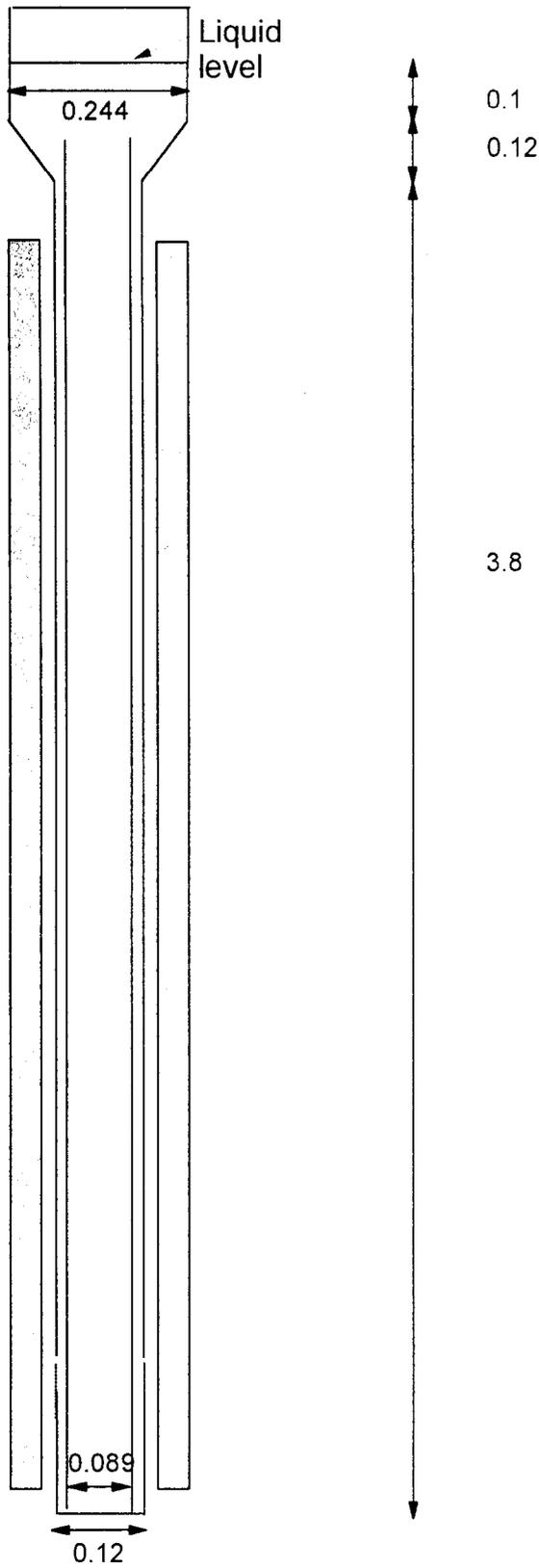
**Figure 3.** Air-lift dimensions for 0.12 m diameter (reactor 2).
