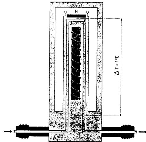
THERMOPILE WITH APPROX. 5000 THERMOELEMENTS
