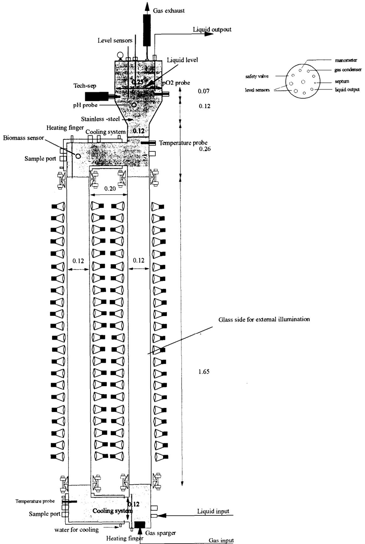
Figure 7. Final proposed airlift design .
