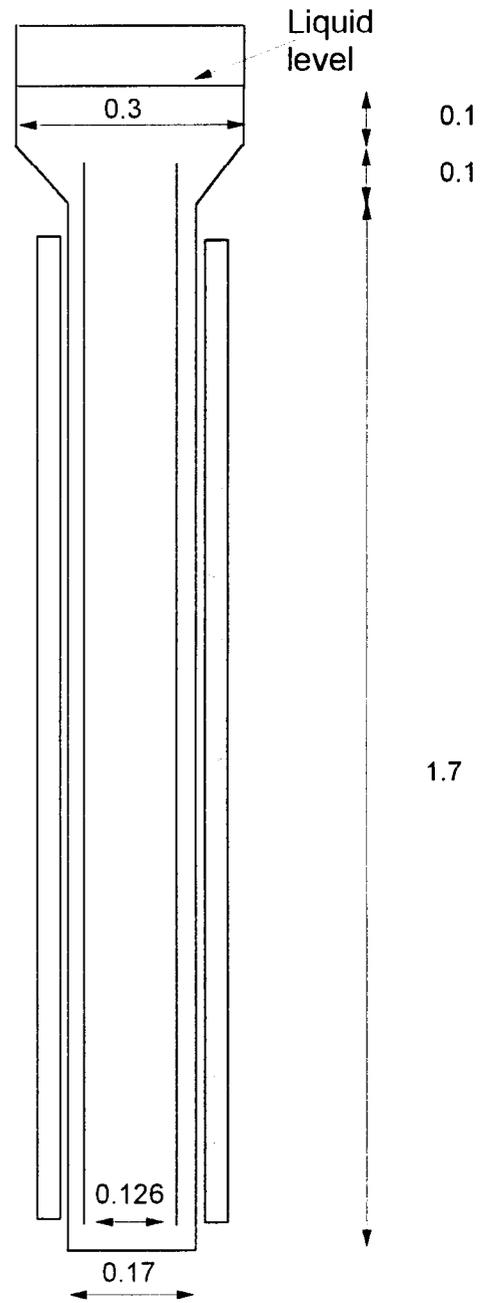
**Figure 4.** Air-lift dimensions for 0.17 m diameter (reactor 3).
