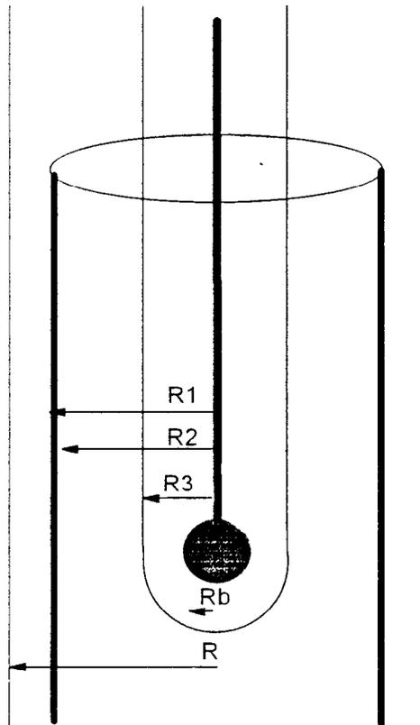
**Figure 6.** Definition of the different radius in the reactor.
