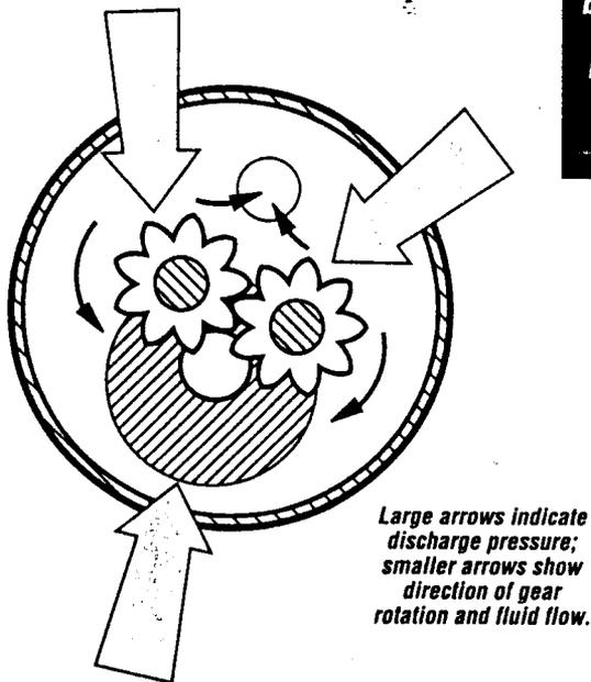
Large arrows indicate discharge pressure; smaller arrows show direction of gear rotation and fluid flow.
