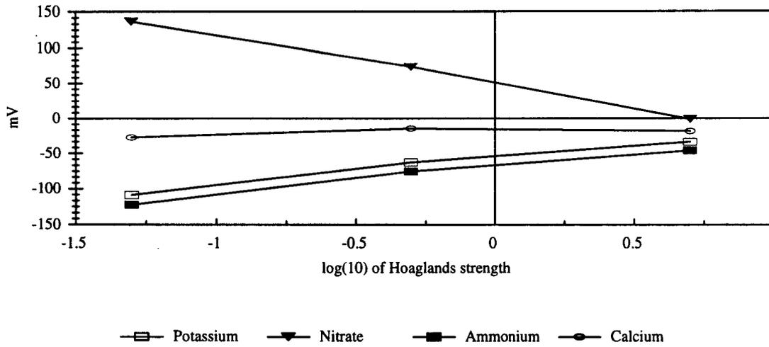
Figure 2. Typical calibration profiles for four ISEs. Electrode output was plotted against the log of the Hoaglands strength, according to Eqn (1). Regression analysis results are presented in Table 1.
