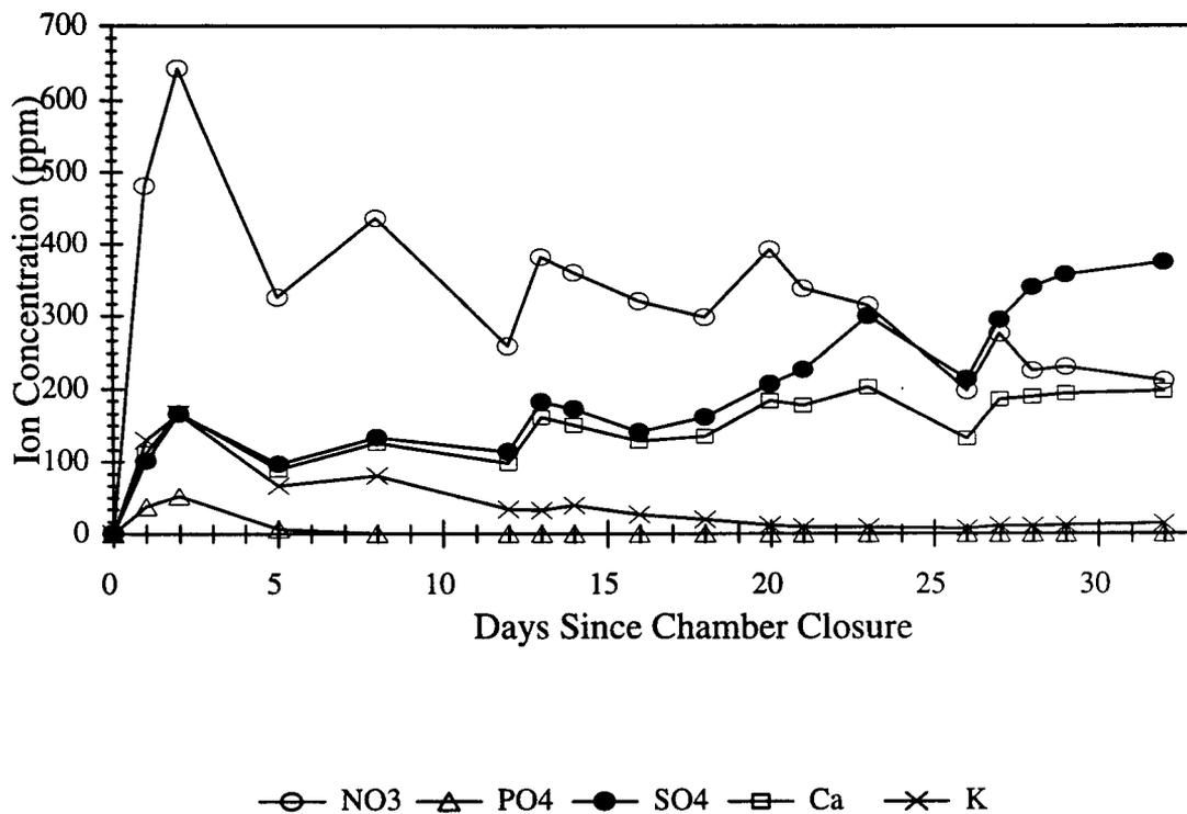
Figure 1. Ion accumulation and depletion patterns in a re-circulating nutrient solution in one of the sealed environment chambers. Concentration estimates were obtained using off-line HPLC with daily sample acquisition. Expected ion concentrations (in ppm) based on a 1/2 x Hoagland's solution are  $\text{NO}_3^- = 310$ ,  $\text{PO}_4^{3-} = 47$ ,  $\text{SO}_4^{2-} = 97$ ,  $\text{Ca}^{2+} = 100$ ,  $\text{K}^+ = 111$ . Stock injections were continuous.
