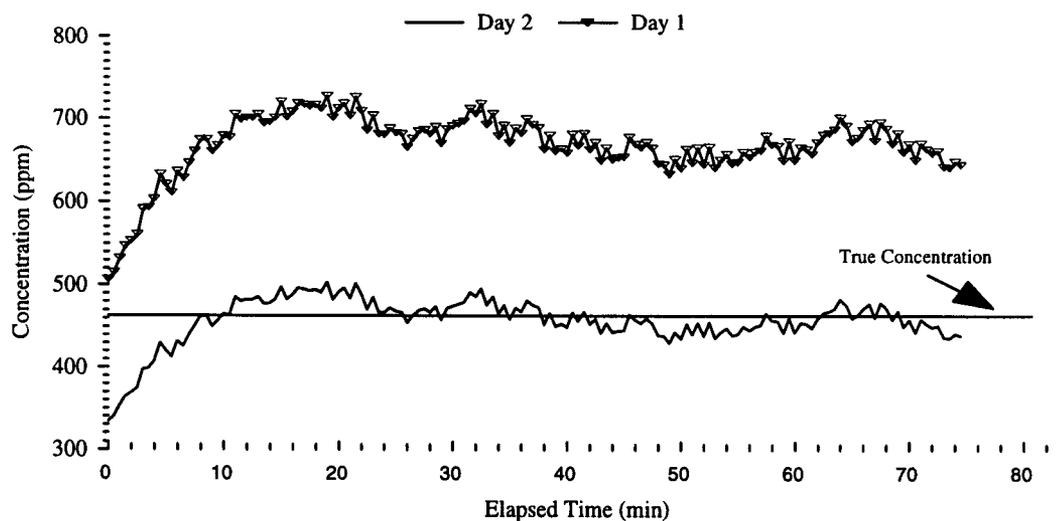
Figure 3. Influence of Nitrate ISE drift on concentration estimates. Nitrate concentration estimates at the end of a 24 hour period were obtained using calibration curves generated at the start and end of the same period (days 1 and 2 respectively). Nitrate electrode output was continuously monitored for over a 1 hour period on each of the two days. Concentration estimates derived from the two calibration sets is plotted as a function of time.
