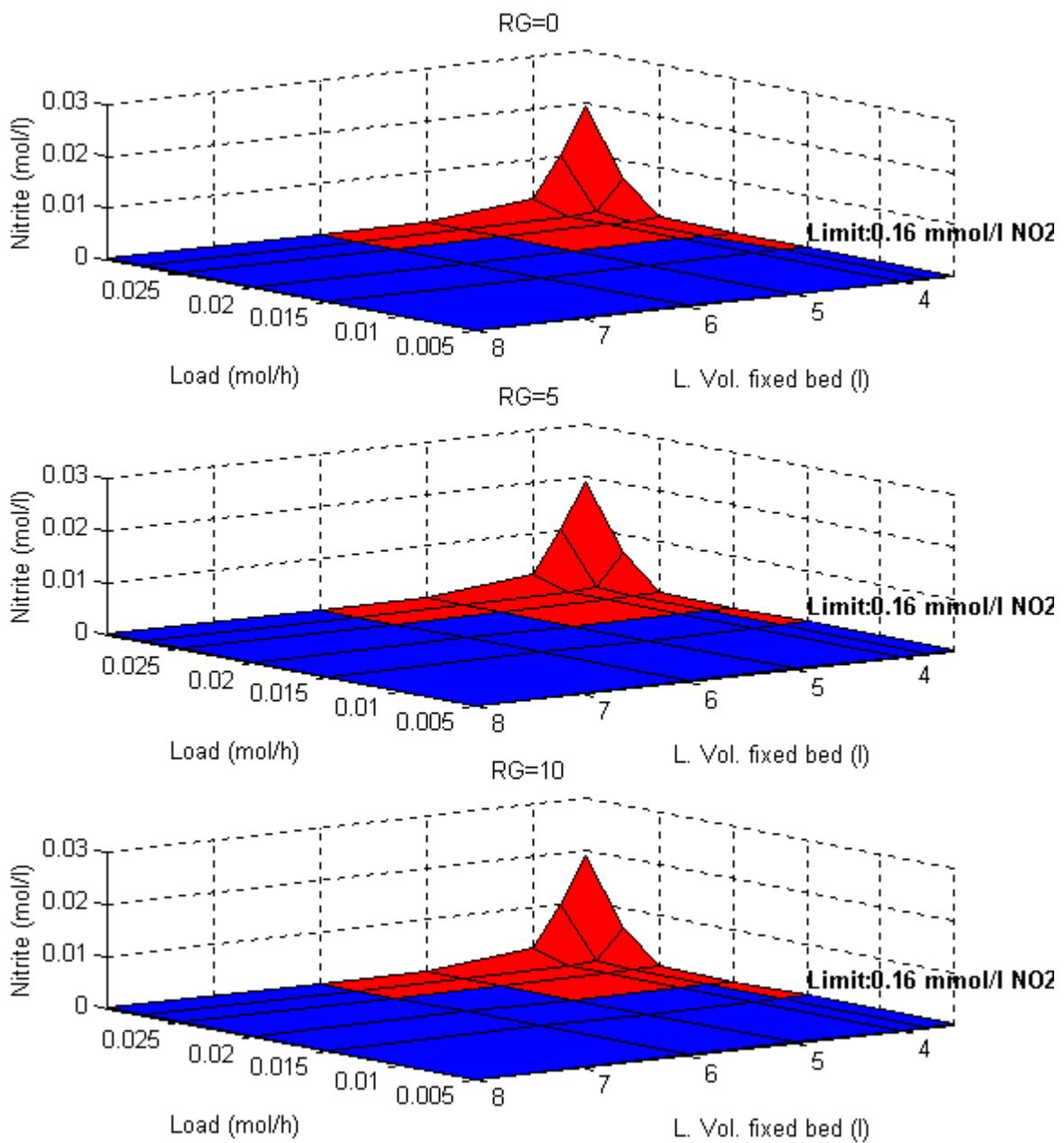
**Figure 2 : Nitrite concentration depending on Volume, Load and  $R_G$**
