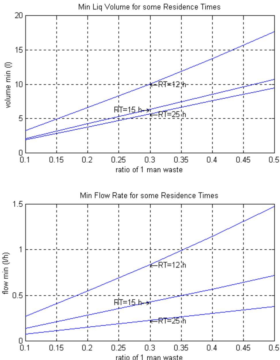
**Figure 4 : Minimum volume and flow rate of Rhodo compartment versus load
