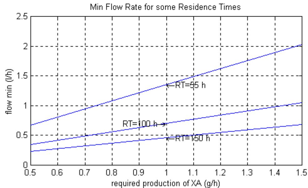
**Figure 5 : Minimum volume and flow rate of Spiru compartment
