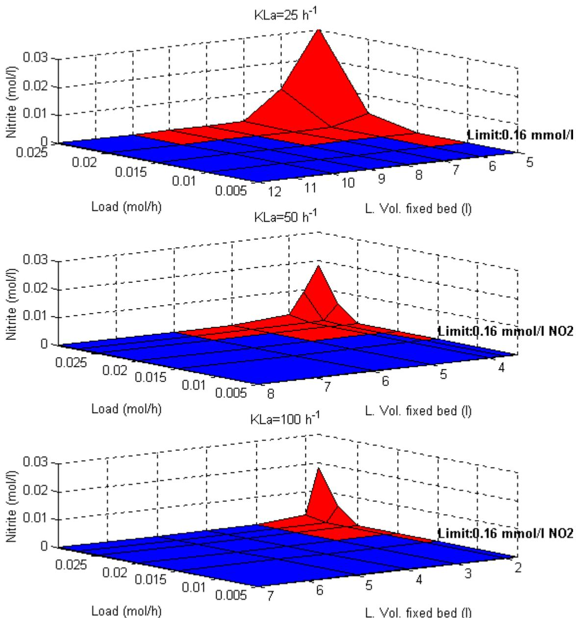
**Figure 1 : Nitrite concentration depending on Volume, Load and  $KLa$**
