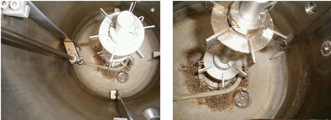
Figure 5.3: Inside Views, Left: Sparger feed pipe, Right: Sparger vent under bottom mixing paddles
