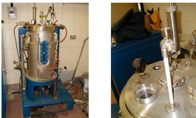
Figure 5.1: Example of an enclosed continuous stirred culture system, a 75 litre fermenter Outside Views, Left: Overall view, Right: Inspection window and feed pipes on cap
