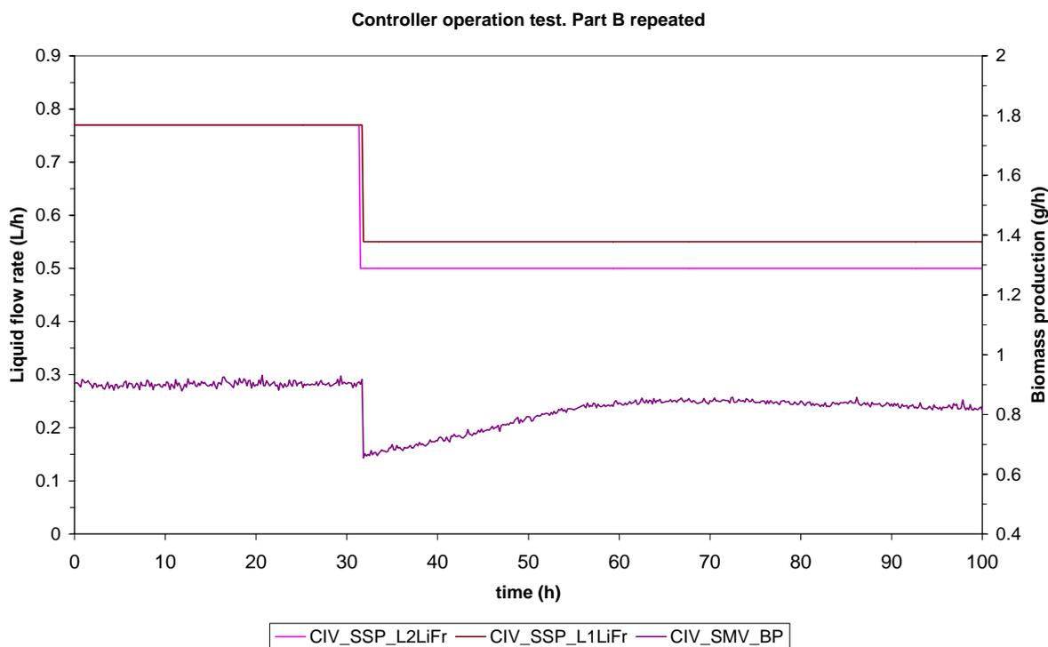
**Figure 12: Values of the liquid flow rate during the repetition of the controller operation test part B. Biomass production is shown as reference with the previous figure.**
