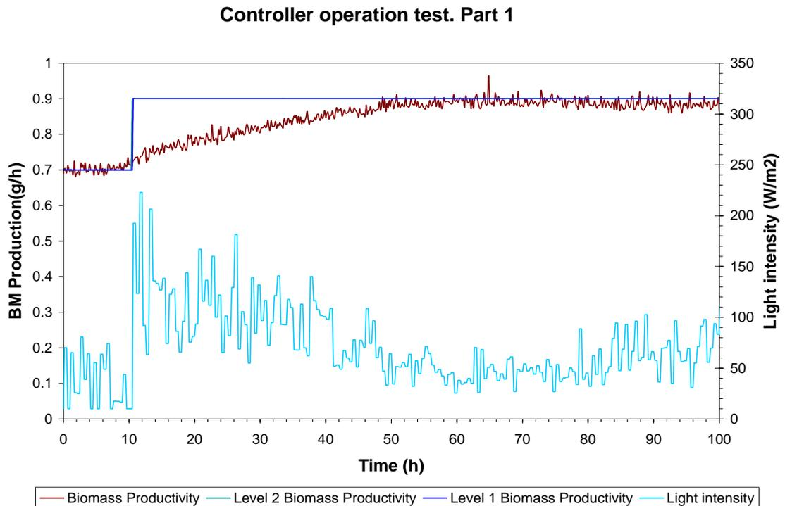
**Figure 7: Evolution of biomass productivity and light intensity during the first part of the controller operation test. Controller biomass productivity level 1 and level 2 values have the same value during all the test.**
