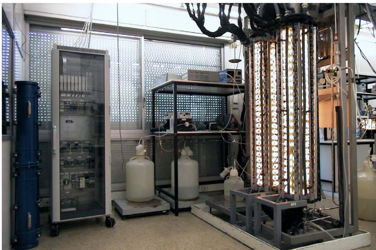
**Figure 1: General view of compartment IVa bioreactor and controller's rack.**
