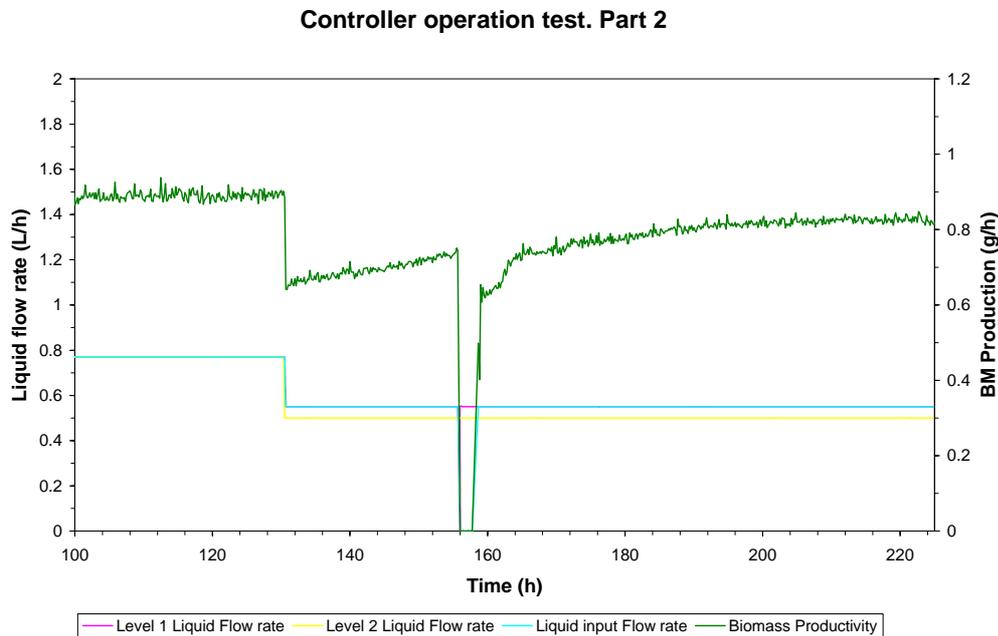
**Figure 10: Values of the liquid flow rate during the first part of the controller operation test part 2. Biomass production is shown as reference with the previous figure.**
