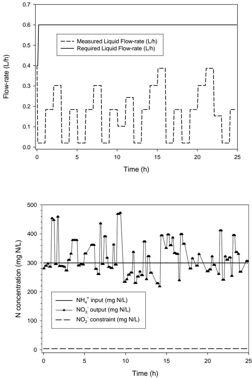
**Figure 14: Long test carried-out in compartment III pilot reactor for the validation of the implementation of the new control system. Requested as well as measured liquid flow-rate are shown in the top graph. In the bottom graph the variation of the nitrite concentration constraint as well as measured nitrate concentration in the effluent are shown.**
