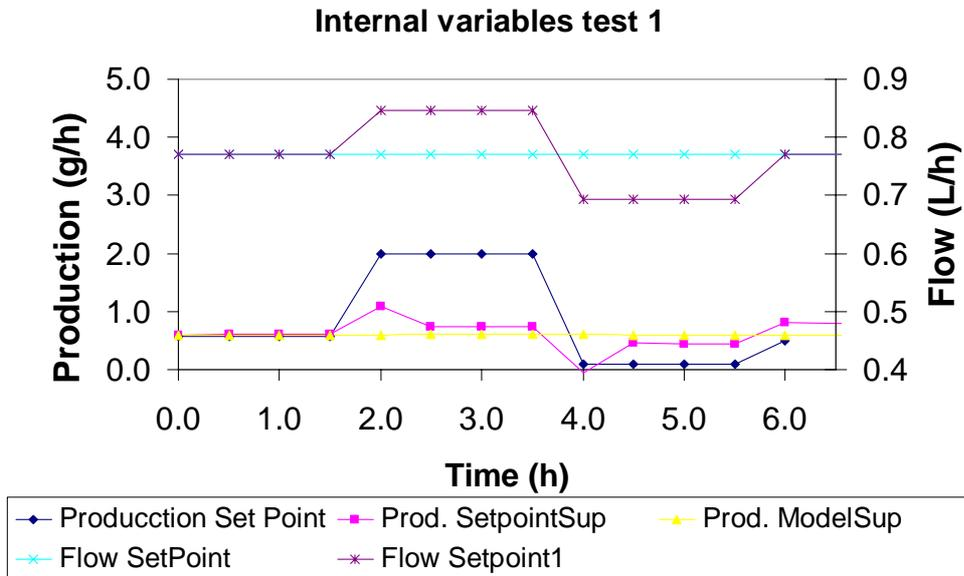
Figure 5: Evolution of variables related to biomass production and liquid flow rate during test 1.
