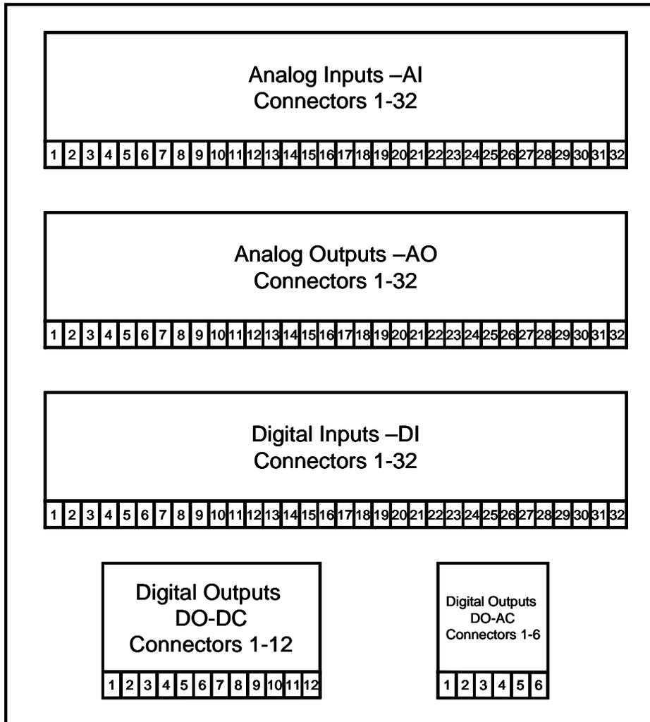
**Figure 4: Scheme of the distribution of the connections inside the auxiliary connection panel for compartment IVa.**
