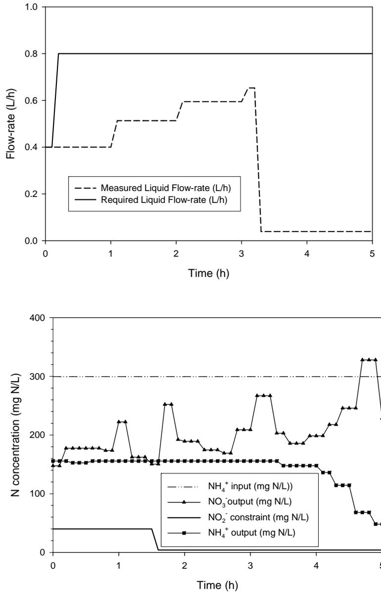
**Figure 13: Short test carried-out in compartment III pilot reactor for the validation of the implementation of the new control system. Requested as well as measured liquid flow-rate are shown in the top graph. In the bottom graph the variation of the nitrite concentration constraint as well as measured ammonium and nitrate concentration in the effluent are shown.**
