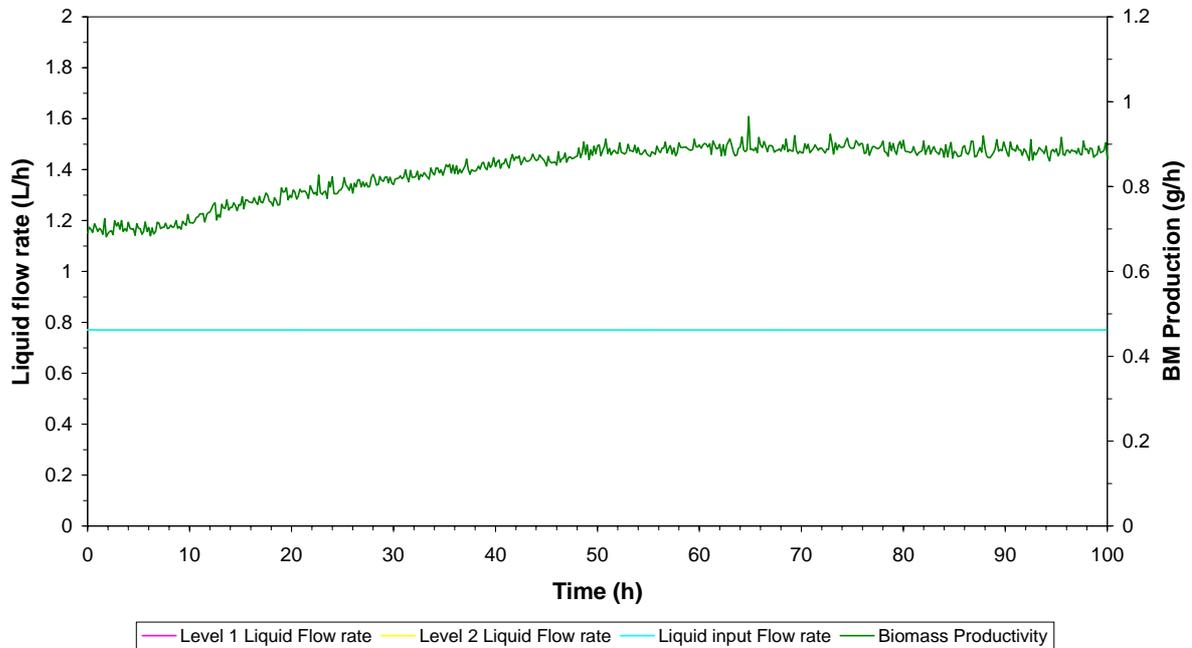
**Figure 8: Values of the liquid flow rate during the first part of the controller operation test. Level 1 and level 2 controller values for the flow rate have the same value as the flow rate and therefore can not be seen. Biomass production is shown as reference with the previous figure.**
