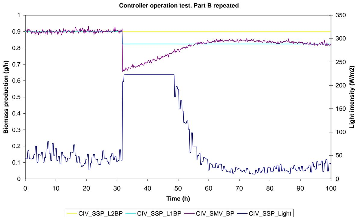
Figure 11: Evolution of biomass productivity and light intensity during the repetition of the controller operation test part B.
