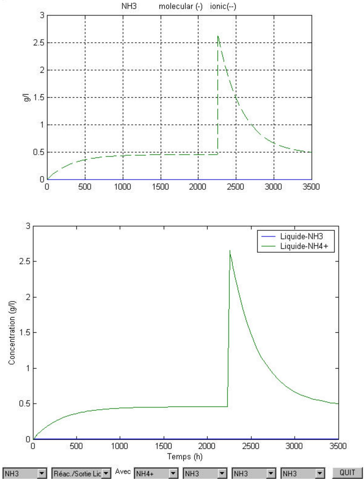
Figure 24. NH3 : Molecular (blue curve) and Ionic (green curve) forms
