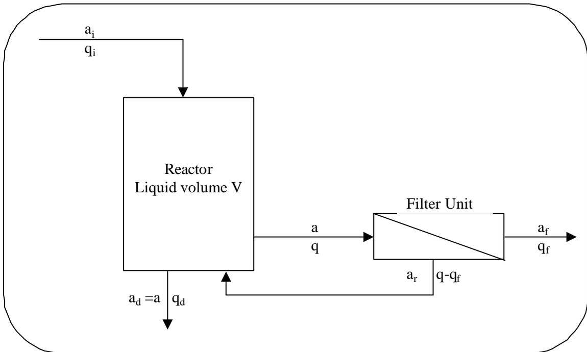
Figure 1. Scheme of the reactor and its filter unit
