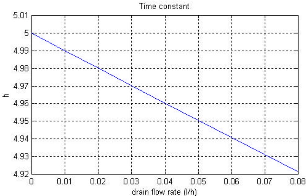
Figure 14. Evolution of time constant in function of drain flow rate
