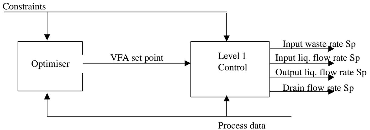
Figure 3. Control architecture: Optimiser and level 1 control
