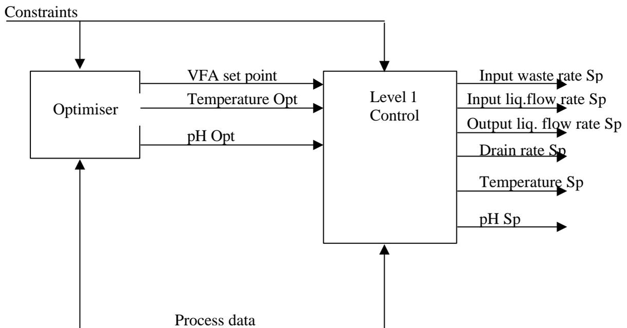
Figure 5. Future control architecture: Optimiser and level 1 control with 2 more freedom degrees (temperature and pH)
