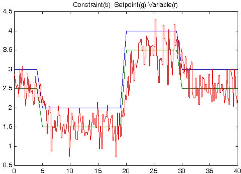
Figure 7. Foreseen test of constraint control (X and Y values are arbitrary).
