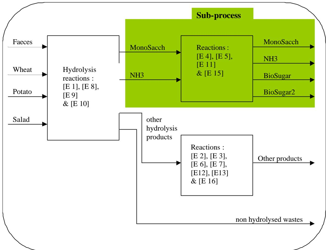
Figure 9. Limits of the studied sub-process (green area) inside the whole process
