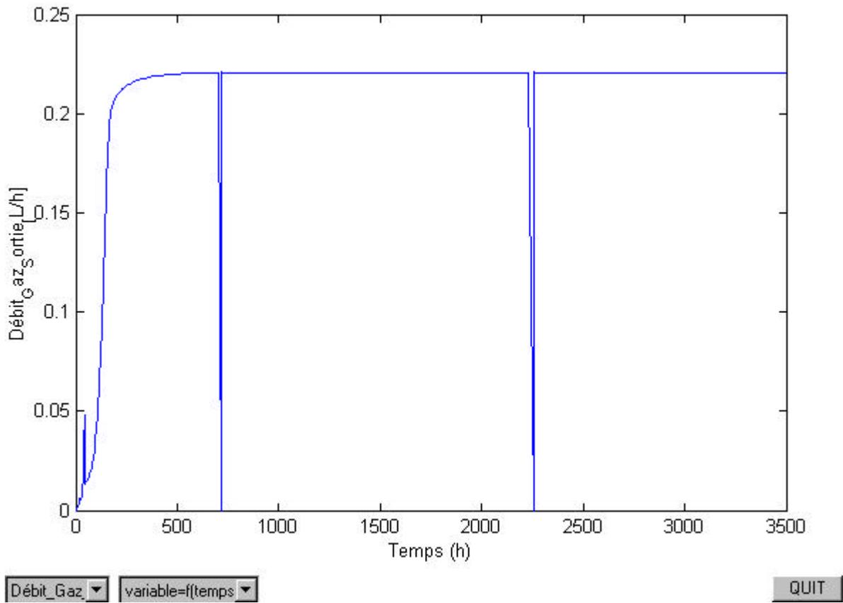
Figure 39. CO2 gas production rate (in l/h at 20 °C and 1 atm)
