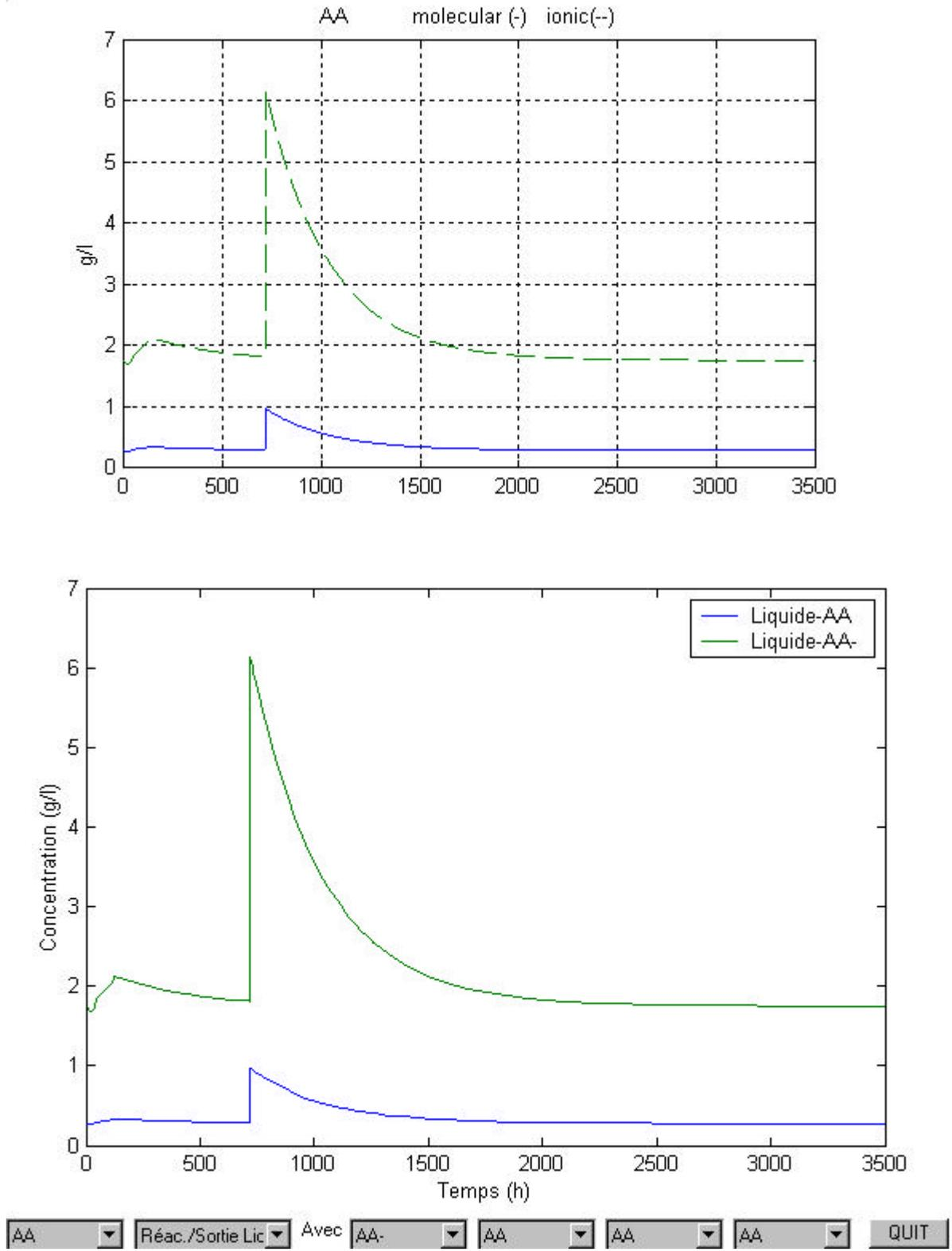
Figure 19. AA: Molecular (blue curve) and Ionic (green curve) forms
