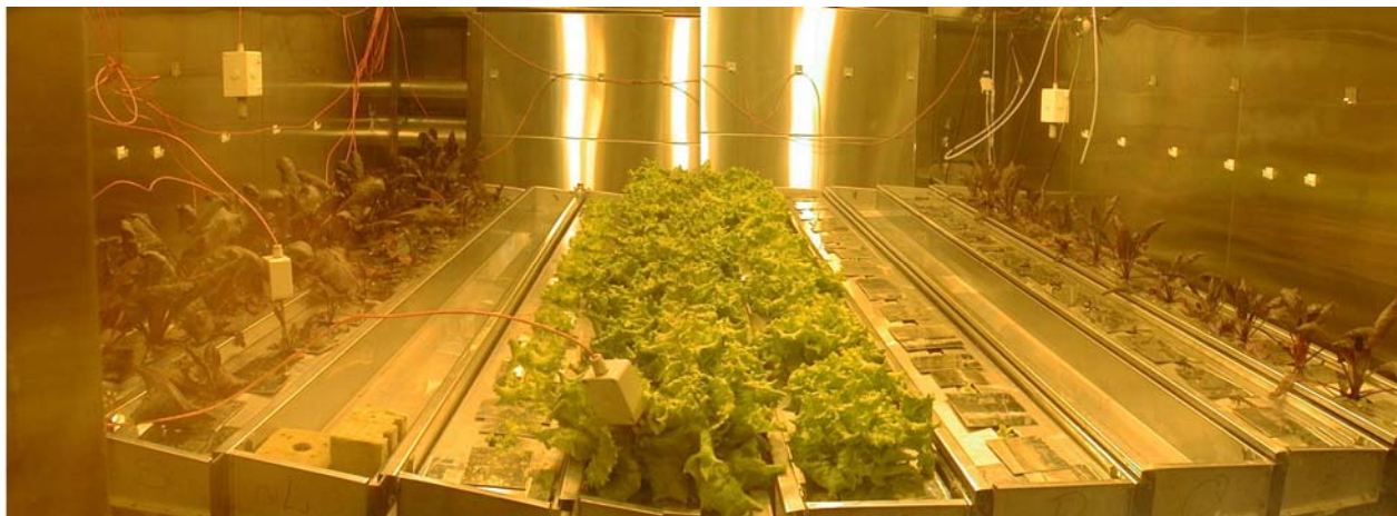
Figure 1 Photograph of one of the SEC-2 Chambers be Used in Phase A studies. The chamber production area is 5m 2 .
