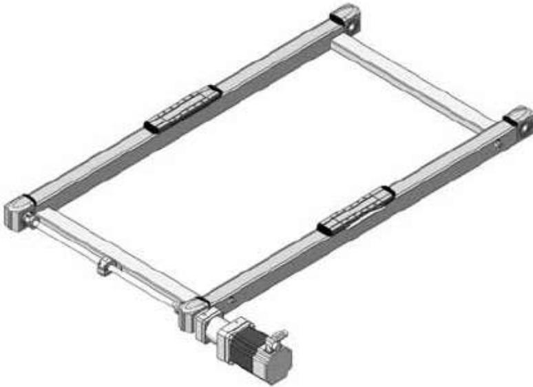
Figure 4: Double axes layout with shaft driven support axis
