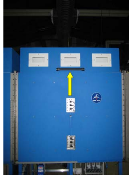
Illustration 3: Location of the lamp loft and lifting handle (yellow arrow).
