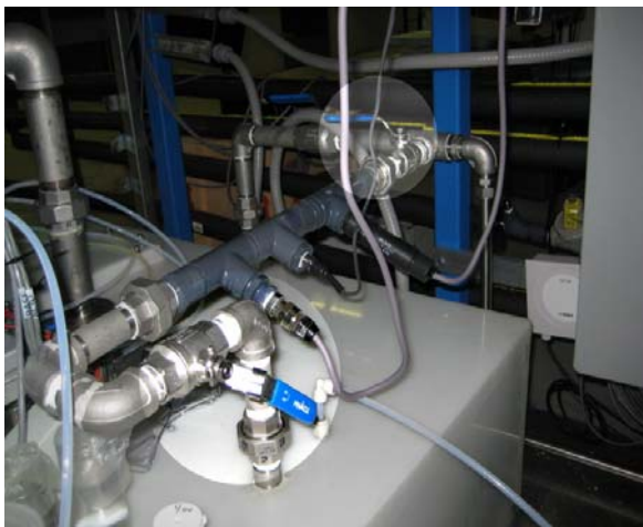
Illustration 1: Location of shut off valves for pH/EC calibration procedure.
