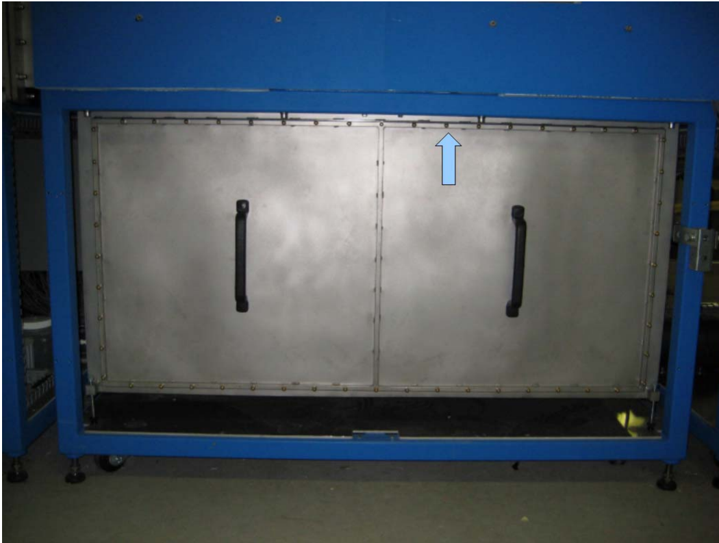
Illustration 5: Blower housing panel. Arrow indicates position of one of the brass plug bolts that secure the panel to the main housing.
