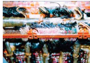
Microbial contamination on a circuit board on Mir
