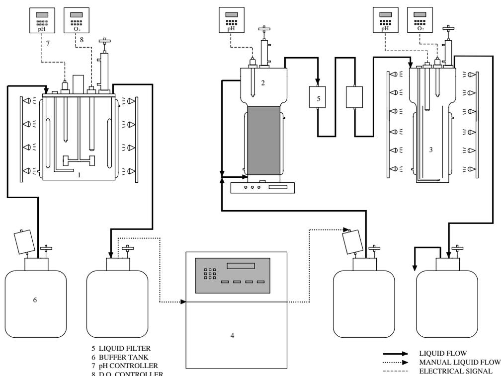
**Figure 2.1.** - Diagram of the experimental set up for the connection of compartments II, III and IVa of MELISSA loop at bench scale.
