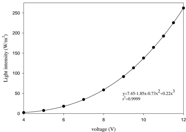
**Figure I.2 .-** Average light intensity supplying different voltages
