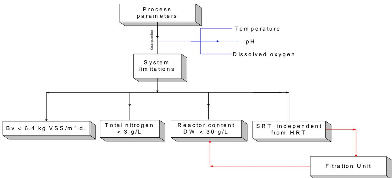
Figure 9. Process requirements for the BWT-Units in Dumont d’Urville and Concordia bases
