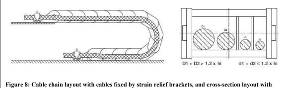
Figure 8: Cable chain layout with cables fixed by strain relief brackets, and cross-section layout with vertical separators
