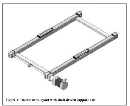
Berger Lahr (Schneider-electric-motion) MAXS2B double axis layout uses a synchronisation connection (Figure 4). This module consists of 2 PAS42BR linear axis of 5m length (Figure 7). The carriages of these 2 parallel axis will carry a single PAS41BR axis of 1m length (Figure 5).
