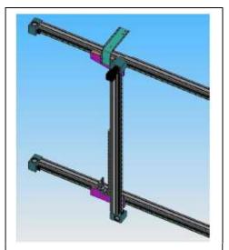
Figure 1: Basic frame of the PSDU workbench demonstrator design: double synchronized axis moving single axis with mobile carriage.
