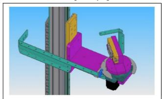
Figure 2: Rotary module with motor of the PSDU workbench demonstrator design
