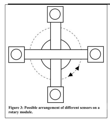
From the preliminary data below, a distance of 100 to 150mm would be sufficient, thus yielding a measuring head with 200 to 300 mm diameter with camera's illumination and other sensors that needs to be rotated depending on the position reached (programming issue dependent on defined grid for imaging). In Figure 3 the camera length and width are set to 50mm.
