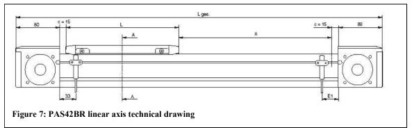
The PAS42BR linear axis has a 60x60mm cross section, a maximal stroke of 5500mm, a typical load of 12kg. Weight per meter of axis: 4.55 kg/m. The carriage has an effective length L2 = 206 (see figure 7).
