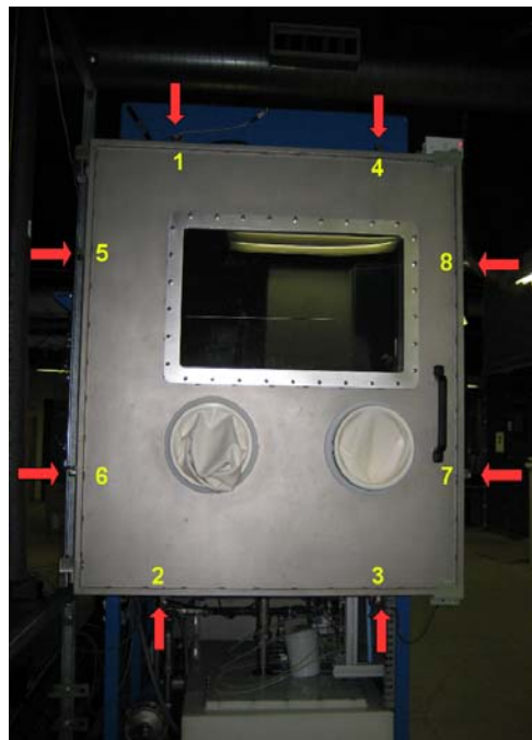
Illustration 6: HPC1 exterior door latch locations. Red arrows indicate latch mechanism locations. Numbers represent the unlatching sequence.
